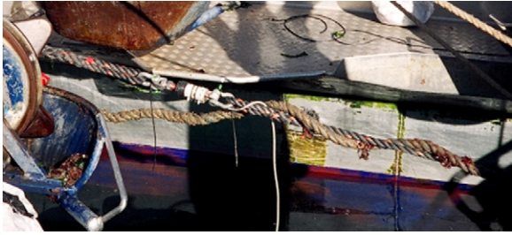
Fig. 6. Load cell mounted inline on a mussel anchor rope.
